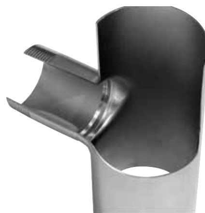
Fig. 9 Manifold with optimised hygienic surface and weldings
